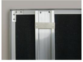
Accessory items for BALANCE wall panel applications typically include strong-back u-clips, which simply fit across strong-backs and are fastened in-place on site as required. Predrilling is recommended to prevent damaging the panel.
